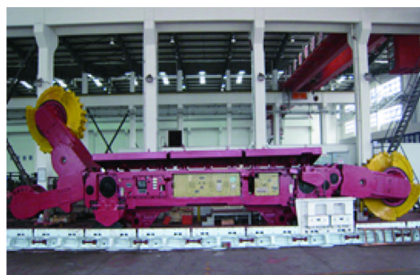
Fig. 42 High efficiency and high reliability electrical haulage shearer
