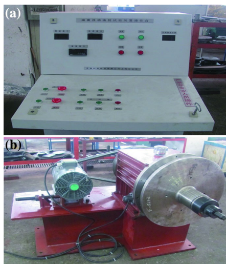
Fig. 52 Floating oil-seal test device. a Electric control console, b mechanical parts of test device
