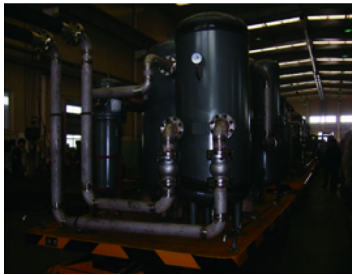
Fig. 68 Nitrogen generator in assembling
